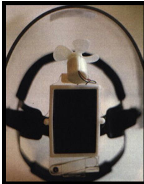
Figure 5: SDL visor with clip on solar fan
