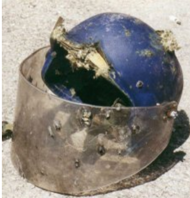
Fragmentation damage to a helmet
