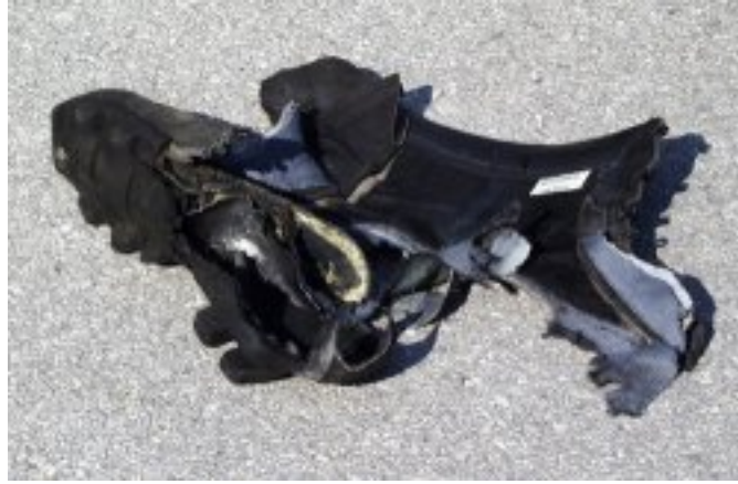
A blast-boot after the wearer stepped on a PMA-3 with 35 g high explosive.
