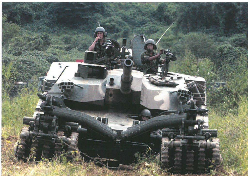
Equipped with a mine detonation device, a South Korean K-1 tank drives across a mine field during training to remove landmines. c/o AP
