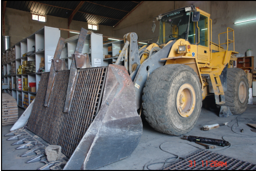
Before. Front end loader before being fitted with armored plating and glass. The machine has already been fitted with a sifter. May 2007.
