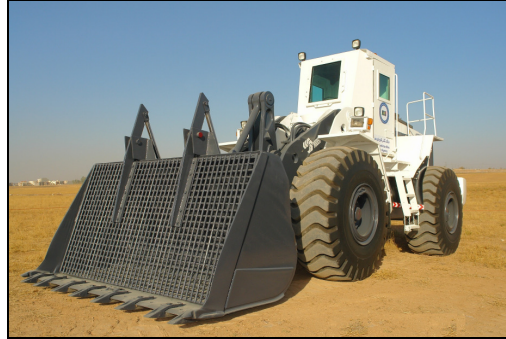
After. The machine has been fitted with armored plates and glass and has just been handed over and delivered to IKMAA. December 2007.
