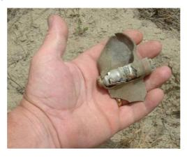
The casing of the mine involved in this accident was intact but may have been hardened by the sun before it became buried, so making it easier to accidentally break open without the case flexing and pushing the liquid explosive into the fuze and making it detonate.
