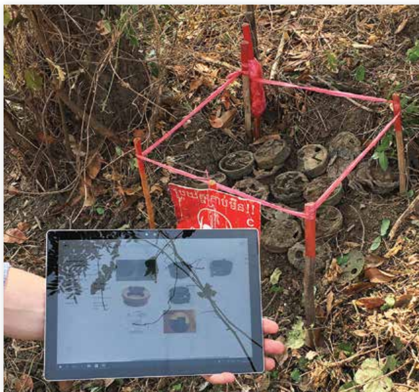
Ordnance objects identified with CORD in the T-IMS ordnance module.
