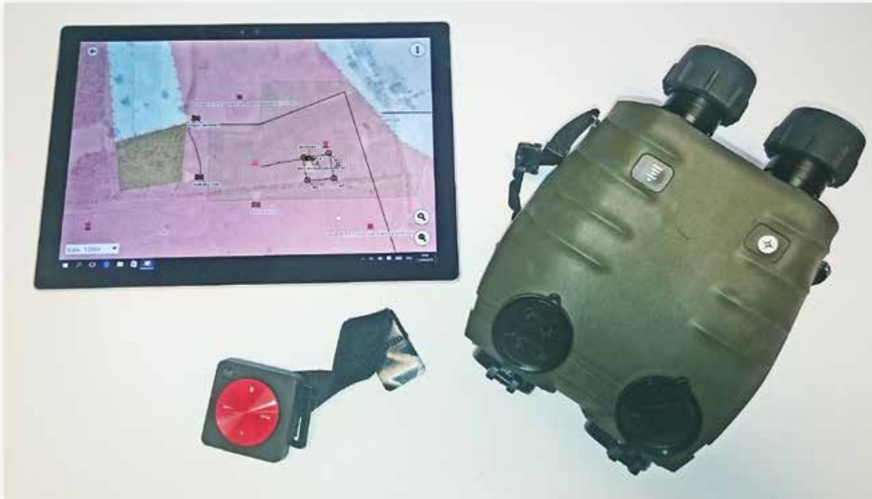
T-IMS with Bluetooth connected GPS and binocular rangefinder. All photos courtesy of © Spinator AB.
