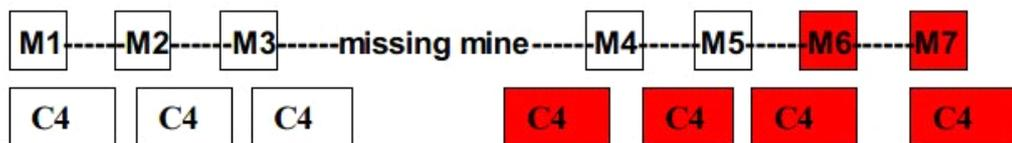
M1 is the first mine, still in place, intact, next to it 100g charge of C4 attached to 1 meter branch of det cord. (see picture 9) [No pictures were made available.]
