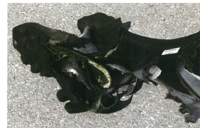
■ A blast-boot after the wearer stepped on a PMA-3 with 35 g high explosive.
