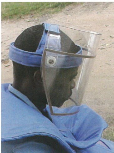
■ (Left to Right) The kind of visor/collar interface that is recommended in IMAS. The long visor is obligatory. The wearer detonated a PROM-1 while cutting vegetation: he died. (The damage was all caused by fragmentation.)
