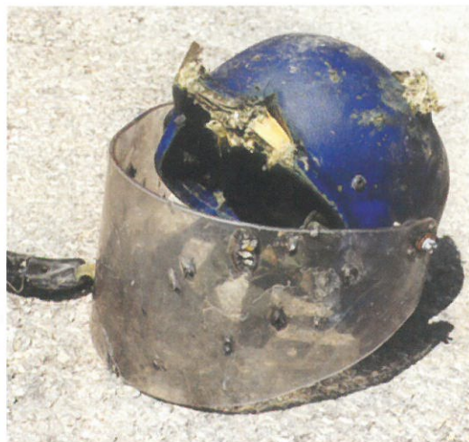
■ (Left to Right) The kind of visor/collar interface that is recommended in IMAS. The long visor is obligatory. The wearer detonated a PROM-1 while cutting vegetation: he died. (The damage was all caused by fragmentation.)
