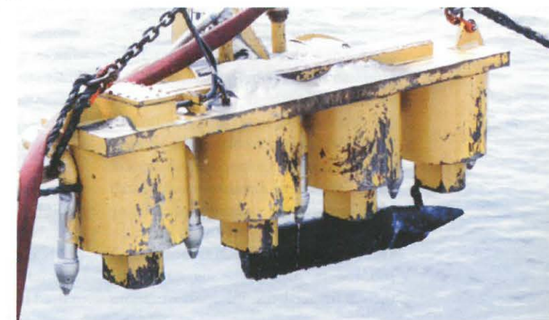
■ Electromagnetic System raising UXO from underwater dumping ground.
