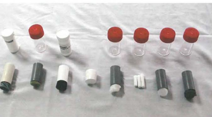
■ APOPO has started trials of different filter material. Seven different materials have so far been tested. The results show relatively good scores on all filters. More testing is required to determine the full potential of these and other materials.
