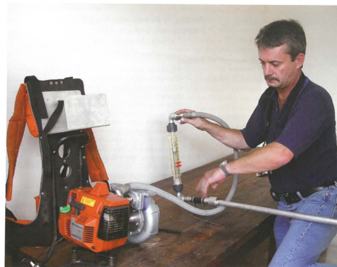
■ Philip Eskeland (IVEMA) demonstrating a modified sampling machine with integrated gauge at the workshop in Tanzania.
