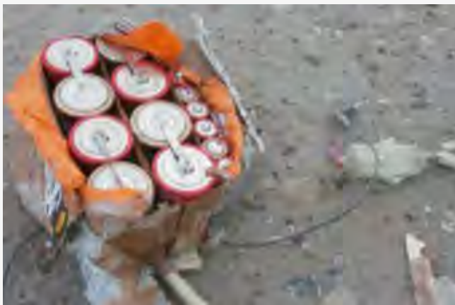
IED Power source consisting of multiple batteries (of different sizes)
