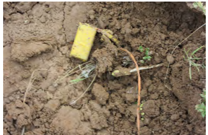
Figure 4. 9V battery used to power improvised landmine pressure plate switch (image credit: FSD).
