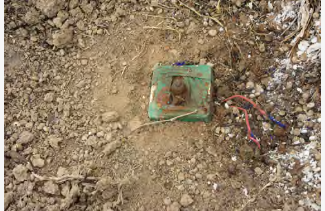
Pressure release switch – Kurdistan (image credit: FSD).
