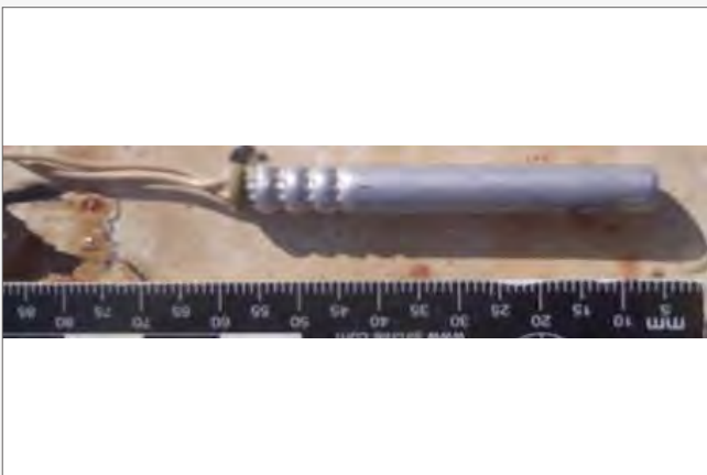
Electric detonator used as IED initiator
