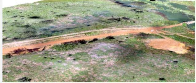
The HALO Trust will use a Swiss-produced [Digger Foundation](#) tilling machine in its clearance operations. The data above—an ArcScene representation of an orthomosaic with the DSM as base heights—was used for slope analysis, which it is thought could prove useful in determining suitable access routes for the machines to reach the sites.
