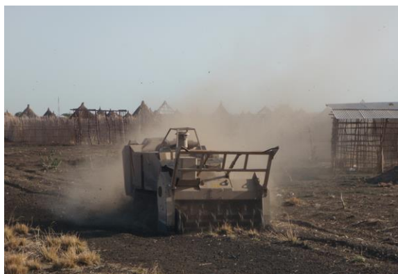
[Mechanical clearance operations with MiniMinewolf 240, MineTech International, Malakal, South Sudan 2010, photo taken by Mikael Bold]
