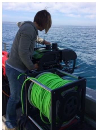
Figure 4. ROV operator placing vLBV300 into the water
