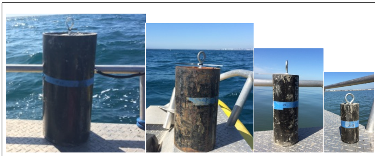
Figure 7. Simulated ERW targets, from left to right: 8-inch, 6-inch, 4-inch, 2-inch diameter steel black pipe filled with low alkali Type II/V cement.
