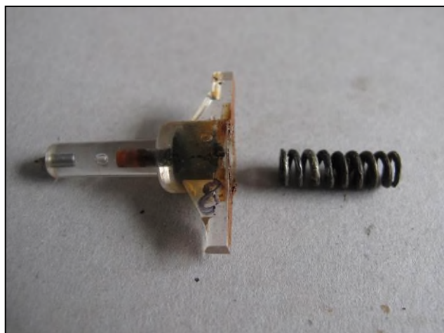
Even when rusted, the steel springs had lost little of their original mass (SB-33 left, SB-81 right)
