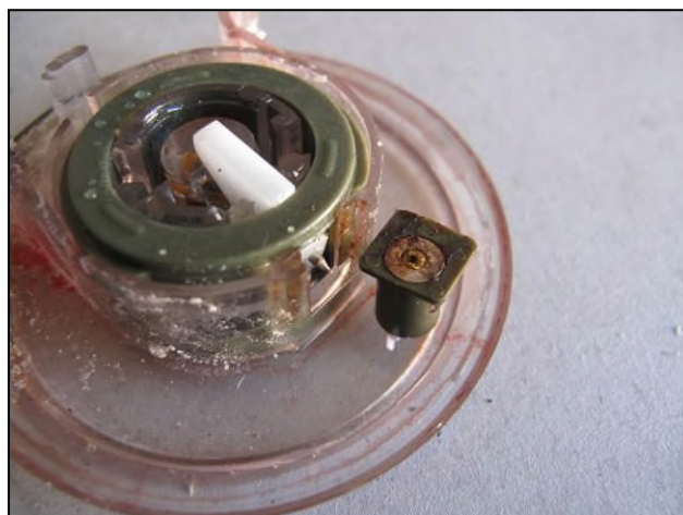
An SB-33 disassembled, showing the pin in the fired position and a hole visible in the detonator
