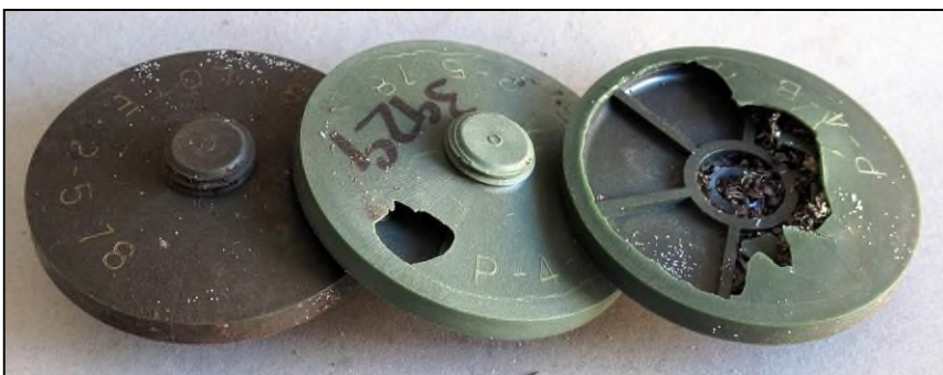
A range of degradation was present among P4B fuze casings
