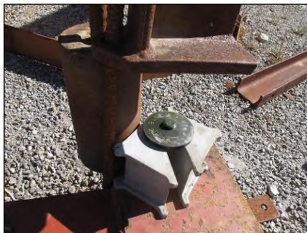
A P4B mine fuze placed on the test rig, ready for the girder to be lowered
