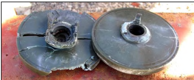
Results from P4B detonator testing. The fuze on the left was one of the few that detonated fully; the one on the right barely had the energy to break the housing and would not have detonated the main charge
