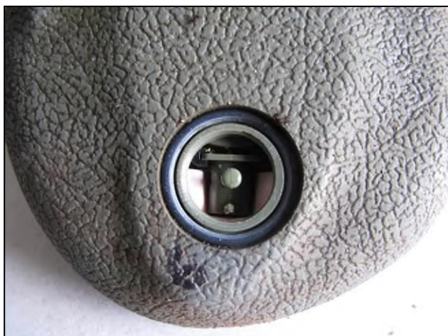
An SB-33 detonator plug removed to reveal the detonator still in position, impaled on the firing pin
