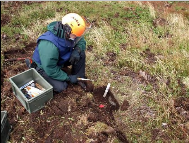
Beginning extraction of an SB-81 AT mine
