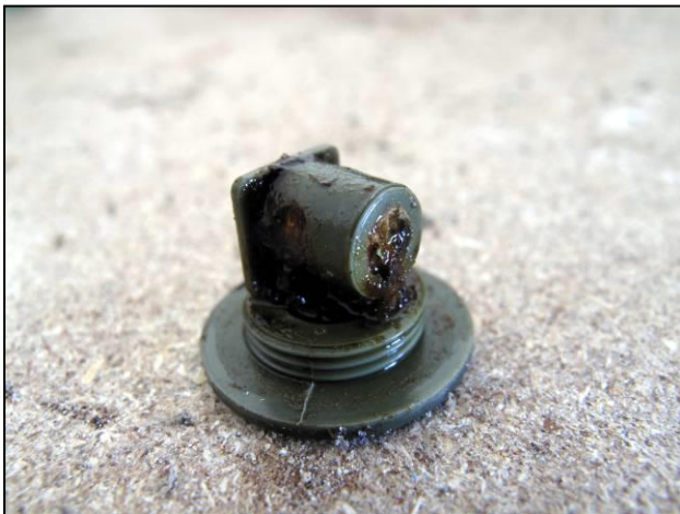
Figure 10: Some detonator capsules did show significant signs of degradation
