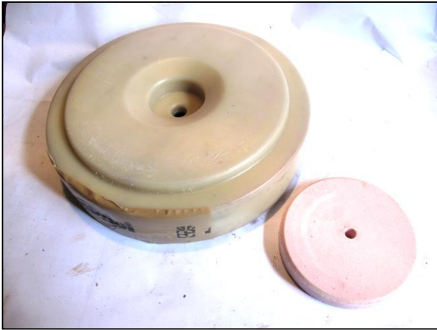
Figure 8: The main charge and booster
