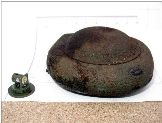
Figure 3: An SB-33 recovered from the Falklands; note the domed profile of the pressure plate
