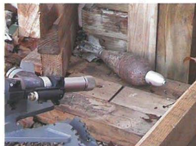
The 20-mm Neutrex firing a 70-grain watershot at an MO81 mortar.
