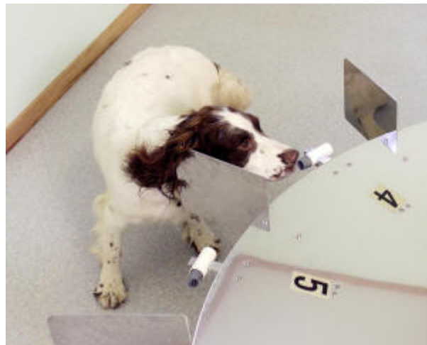
Figure 1: Circular array presentation of the filters. Dogs were trained to circle the array once, but some overlap at the start and end of the circle sometimes occurred. During testing, the array presented 12 filters.
