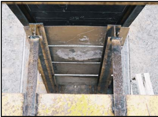
Figure 17. Witness Plates Before Blast
