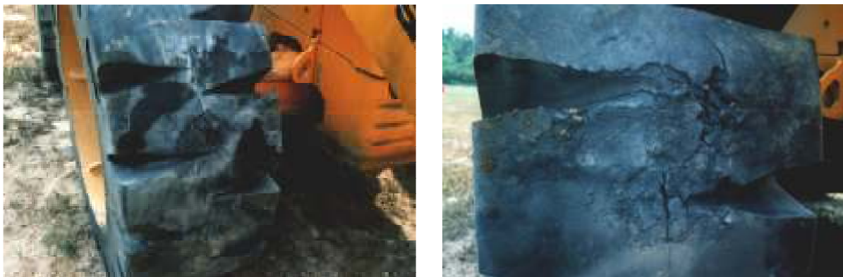
Figure 19. Tire Damage From ½-lb (left) and 1-lb (right) Mine Charge
