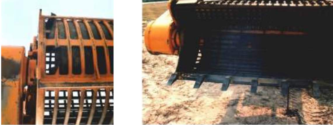
Figure 17. Blast Test Damage to Steel Liner
