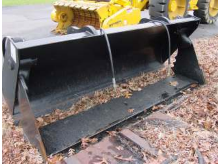
Figure 15. The 6-in-1 Bucket
