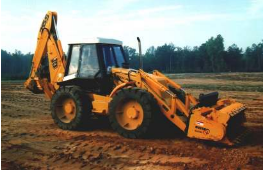
Figure 1. Improved Backhoe With HPL 800 S ROTAR ®
