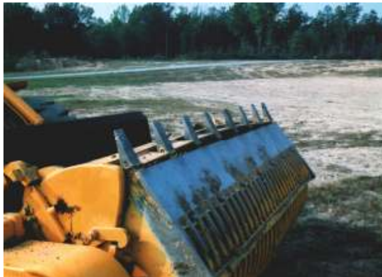
Figure 16. Blast Distortion (Bowing) to ROTAR ®
