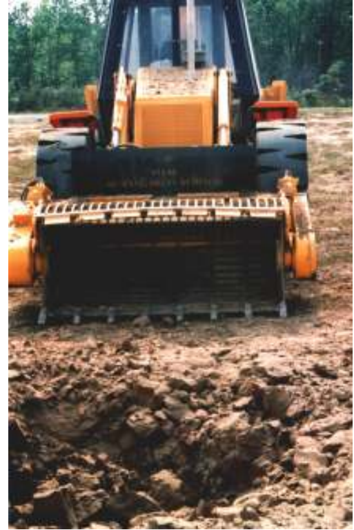
Figure 21. Improved Backhoe After AT Mine Detonation
