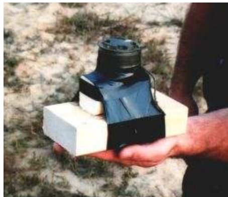
Figure 18. A 1-lb Explosive Charge
