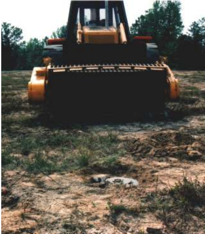
Figure 20. Improved Backhoe Before AT Mine Detonation
