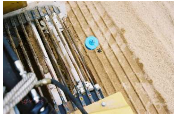
Figure A-18: Mine Deposited at Side of Sifter
