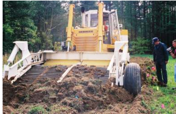
Figure A-14: HLS Sifting Light Clay and Sod
