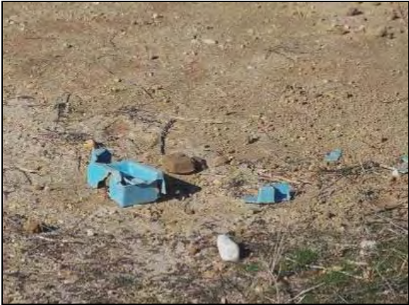
Figure 45: Box Mine Broken in Pieces by Planer, Test Site C (Pieces Recovered by Test Personnel)
