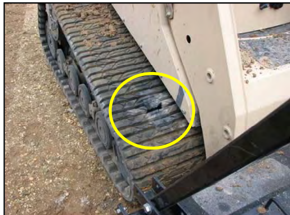
Figure 67: Damage to Track Exterior, Mine C
