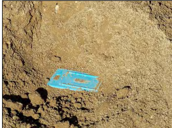
Figure 46: Box Mine Untouched by Planer, Test Site C (Uncovered by Personnel for Photo)
