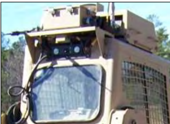
Figure 4: Vehicle-Mounted Remote Transmit/Receive Antennas and Electronics Box
