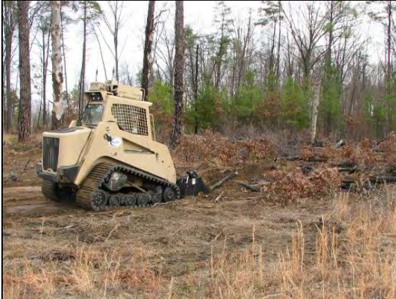
Figure 36: Scooping Small Debris with the 4-in-1 Bucket
