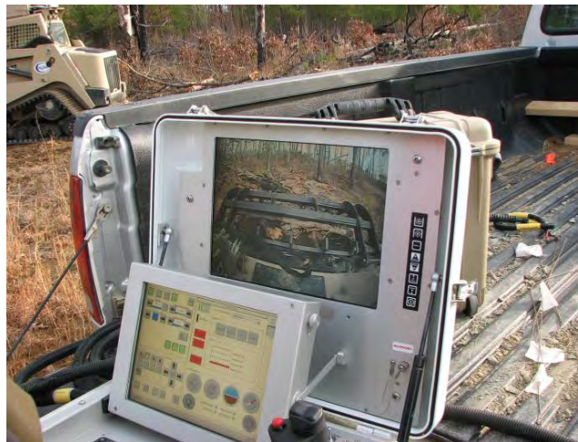
Figure 35: Remotely Controlling Nemesis with Operator Control Unit
