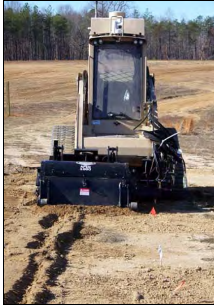
Figure 39: Cold Planer Attached to Nemesis
