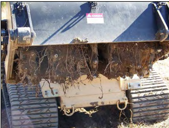
Figure 53: Dirt and Vegetation Accumulation Inside Planer
