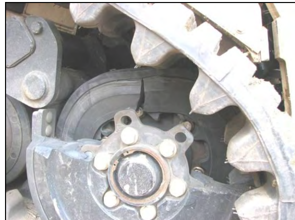
Figure 69: Damage to Outer and Inner Wheel, Mine C
