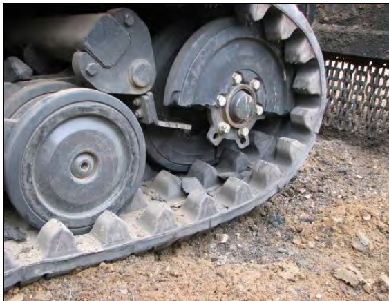
Figure 68: Damage to Outer Wheel, Mine C
