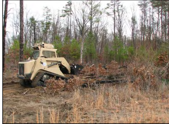
Figure 37: Scooping Small Debris with the 4-in-1 Bucket
