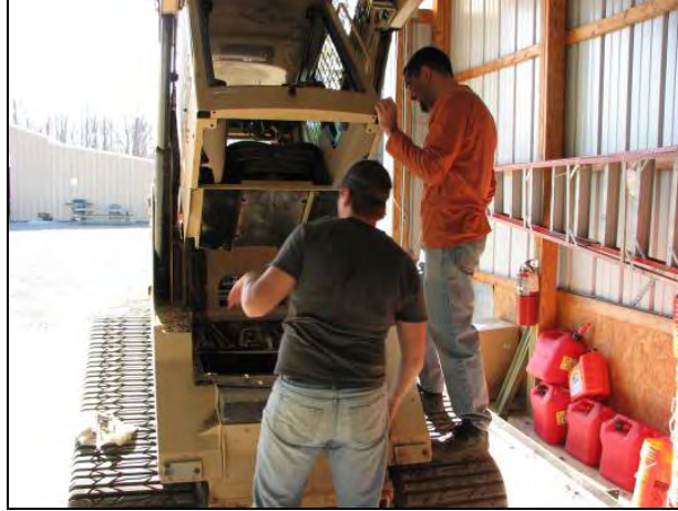
Figure 21: Cab Raised for Maintenance Inspection
