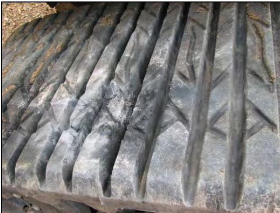
Figure 64: Damage to Track Exterior, Mine A
