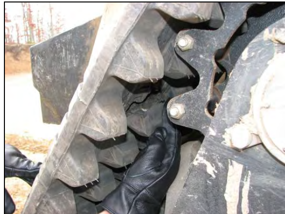
Figure 65: Damage to Track Interior, Mine A
