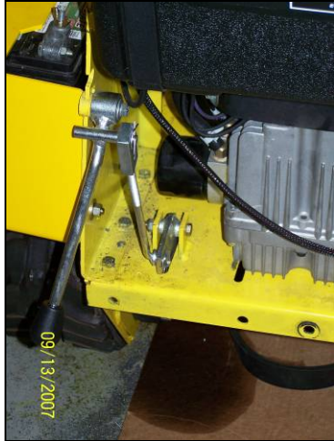
Figure 8: Manual Cutter Engaging Lever Before Modifications
