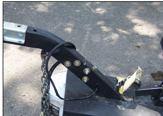
Figure 34: Trailer Connecting End, After Modifications
