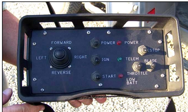
Figure 10: Hand-held Remote Control Device
