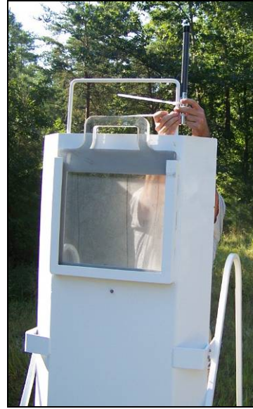
Figure 25: Mounting Remote Antenna to Operator Shield
