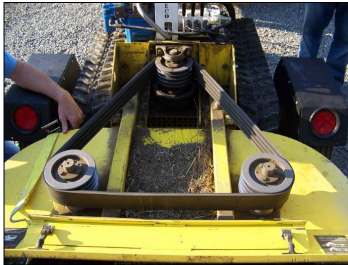
Figure 28: Cutting Blade Belt (Top Cover Removed for This Photo)
