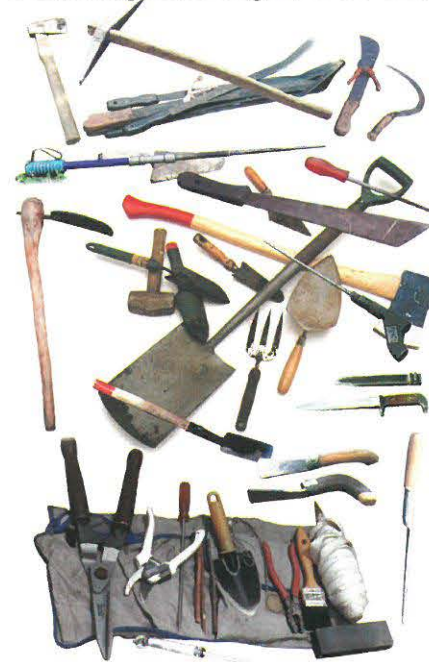
■ (Left) Commonly used demining tools—most of which are unsafe. (Below) Inappropriate tools that have featured in accidents.
