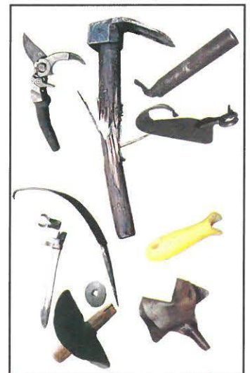
■ (Left) Commonly used demining tools—most of which are unsafe. (Below) Inappropriate tools that have featured in accidents.
