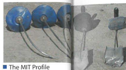
■ The Mini-spade after blast tests
