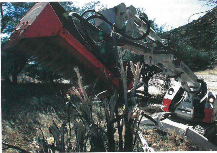
■ (Left) The first mini-mulcher during a trial at the end of May 2002. (Below) The MgM Tree shear carries a large trunk out of the mined area.
