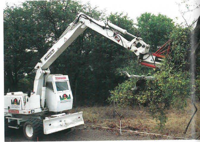
■ (Left) The first mini-mulcher during a trial at the end of May 2002. (Below) The MgM Tree shear carries a large trunk out of the mined area.
