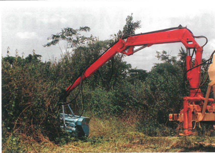
■ MgM mulcher mounted on the back of an armoured "Wolf."
