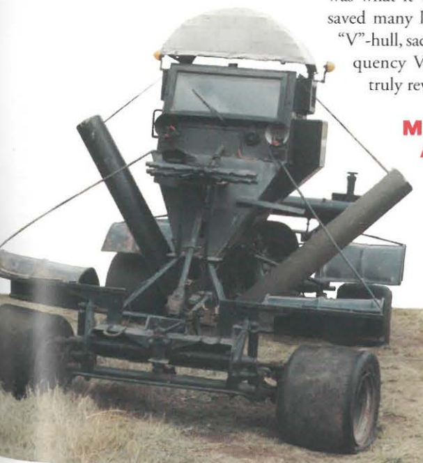
■ The Pookie: a single-seat mine-resistant mine-detection vehicle.
