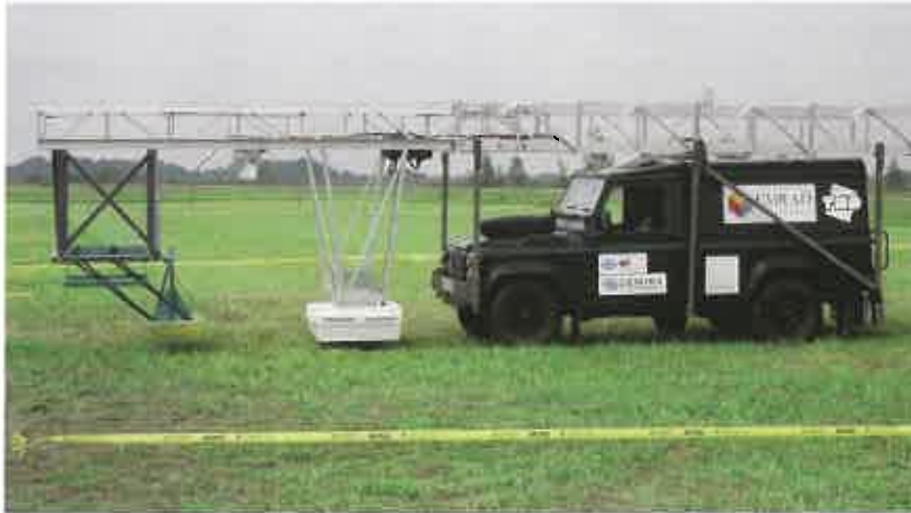
The EC has long supported research and development of new mine action technologies like the tool shown above, a multi-sensor that combines the powers of ground-penetrating radar, infrared cameras and metal detectors.
