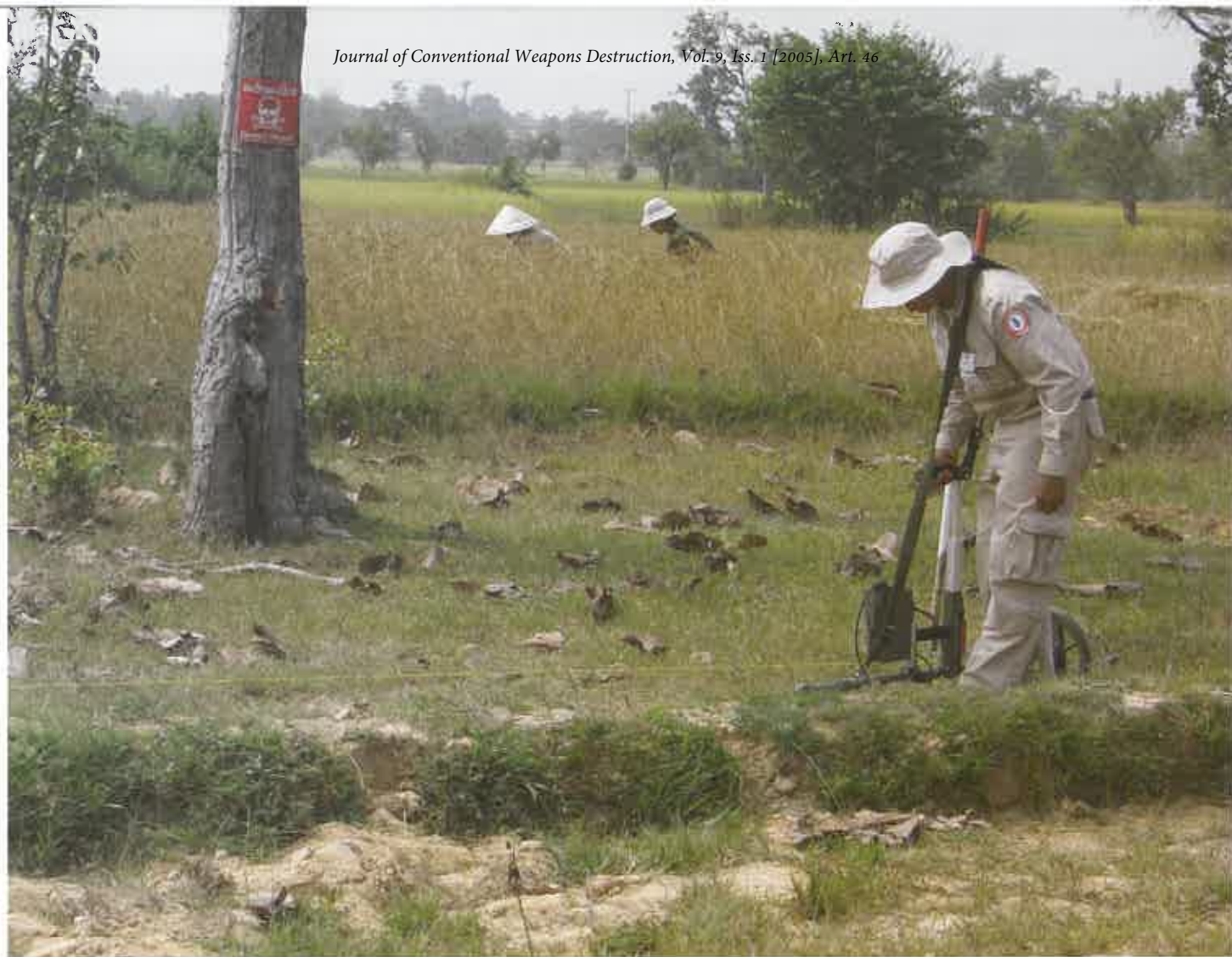
Reliability test of a CEIA Mil D-1 DS detector at Test Site 1, Saravan, Laos.
