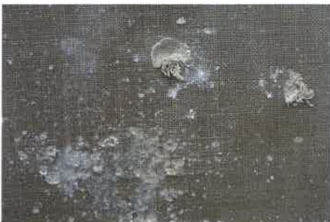
FIGURE 7 Flax composite front side damage after detonation of 70 g of C4 explosives.
