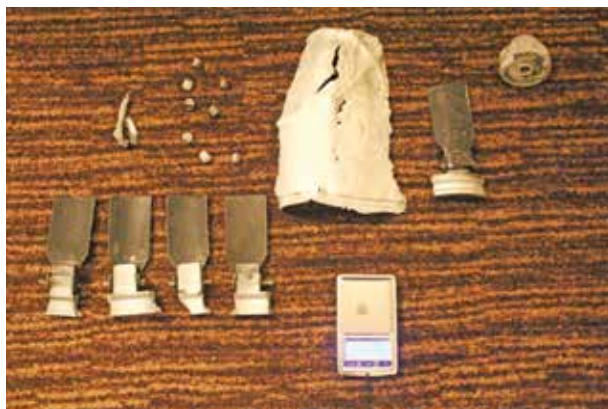
Image 6. Fragmentation from a 9N210 submunition collected at the scene of a cluster munition strike in Donetsk, October 2014. It is important to try to corroborate submunition impact patterns with associated fragmentation when possible. Photo courtesy of Harriet Salem.
