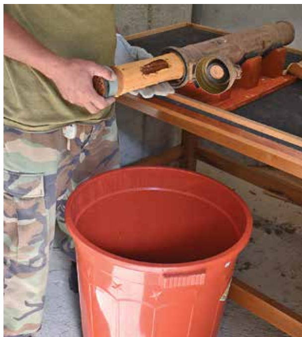
Inspection of ammunition in the Ammunition Processing Area: A typical condition of a propellant charge degrading over time, which results in the ammunition being unserviceable and in need of disposal.
