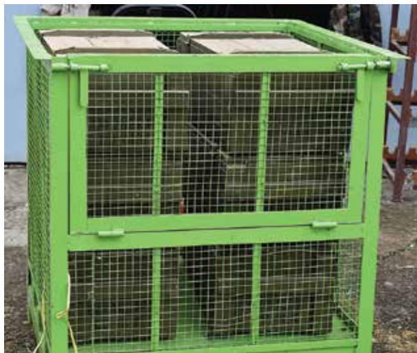
Basic items such as this locally designed and produced cage pallet help with safe movement of loose boxes of ammunition, where items such as banding equipment are not viable in low-income countries as a sustainable solution.
