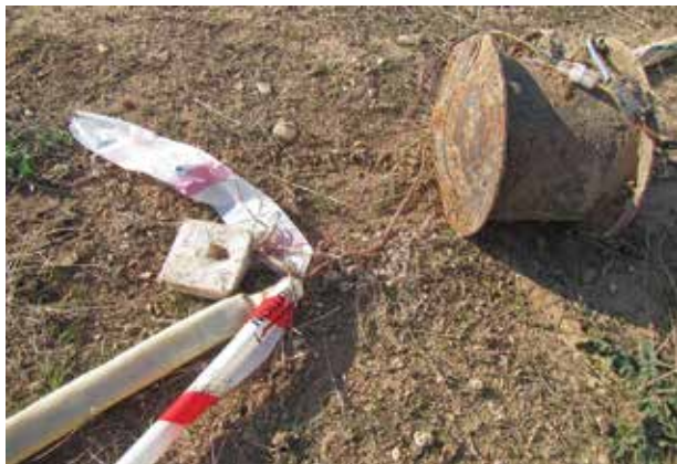
The same PPIED after neutralization. Note the square, white electronic anti-lift device on the left.
