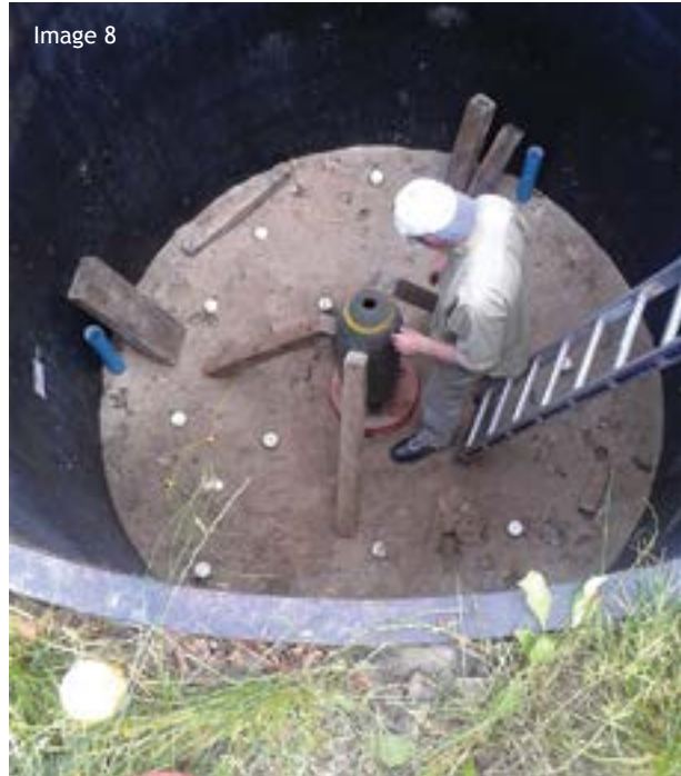
Images 8 and 9. Data collection at a borehole test pit. A 3 m deep test pit is used to collect measurements of ordnance that are then added to a reference library of target polarizabilities. The test pit is also used to collect QC measurements that verify classification processing.
