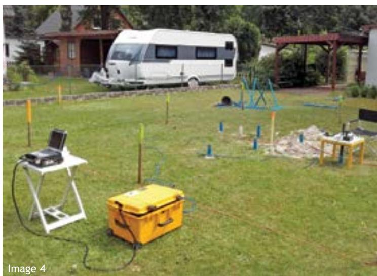
Images 1-4 (left). Examples of borehole EM surveys carried out at urban sites in Germany (blue PVC tubes are borehole casings). The red cable, most evident in Image 2, shows the transmitter cable, and wooden stakes are used to position loop corners. The yellow table visible in Image 3 is used to orient and lock the grey vertical shaft, which has the fluxgate magnetometer at its downhole end.
