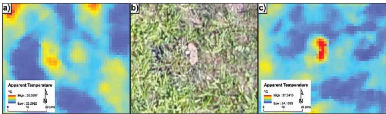
Figure 6. Apparent temperature from (a) 8:16-8:23 AM flight and (c) 9:18-9:24 AM flight before and after direct heating from sunlight, and (b) visible light color photos over the same area.
