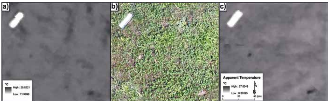
Figure 7. Close up of a single PFM-1 mine apparent temperature at (a) 8:16-8:23 AM flight and (c) 9:18-9:24 AM flight, and (b) visible light color photos over the same area. Aluminum KSF-1 casing can be seen in the top left and PFM-1 landmine in the bottom right.
