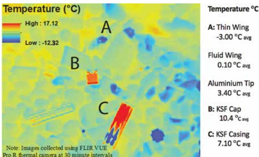
Figure 10. Trial 2, differential apparent thermal inertia taken every 30 minutes of PFM-1s and KSF-1 casing in cobble environment S4 eptember 2017 ( $^{\circ}\text{C}/\text{hour}$ ).
