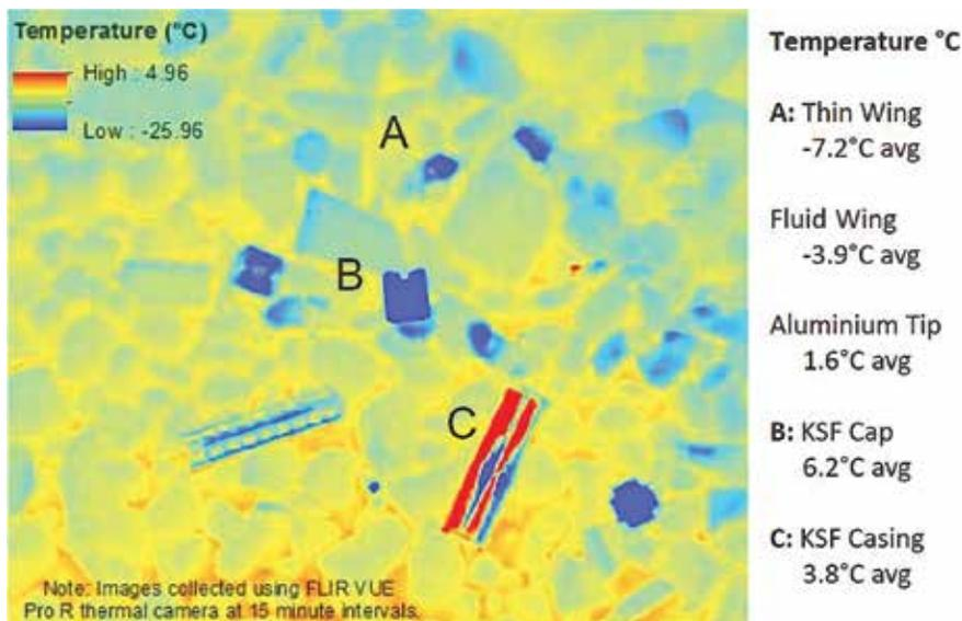
Figure 9. Trial 1, differential apparent thermal inertia taken every 15 minutes of PFM-1s and KSF-1 casing in cobble environment 1 September 2017 ( $^{\circ}\text{C}/\text{hour}$ ).
