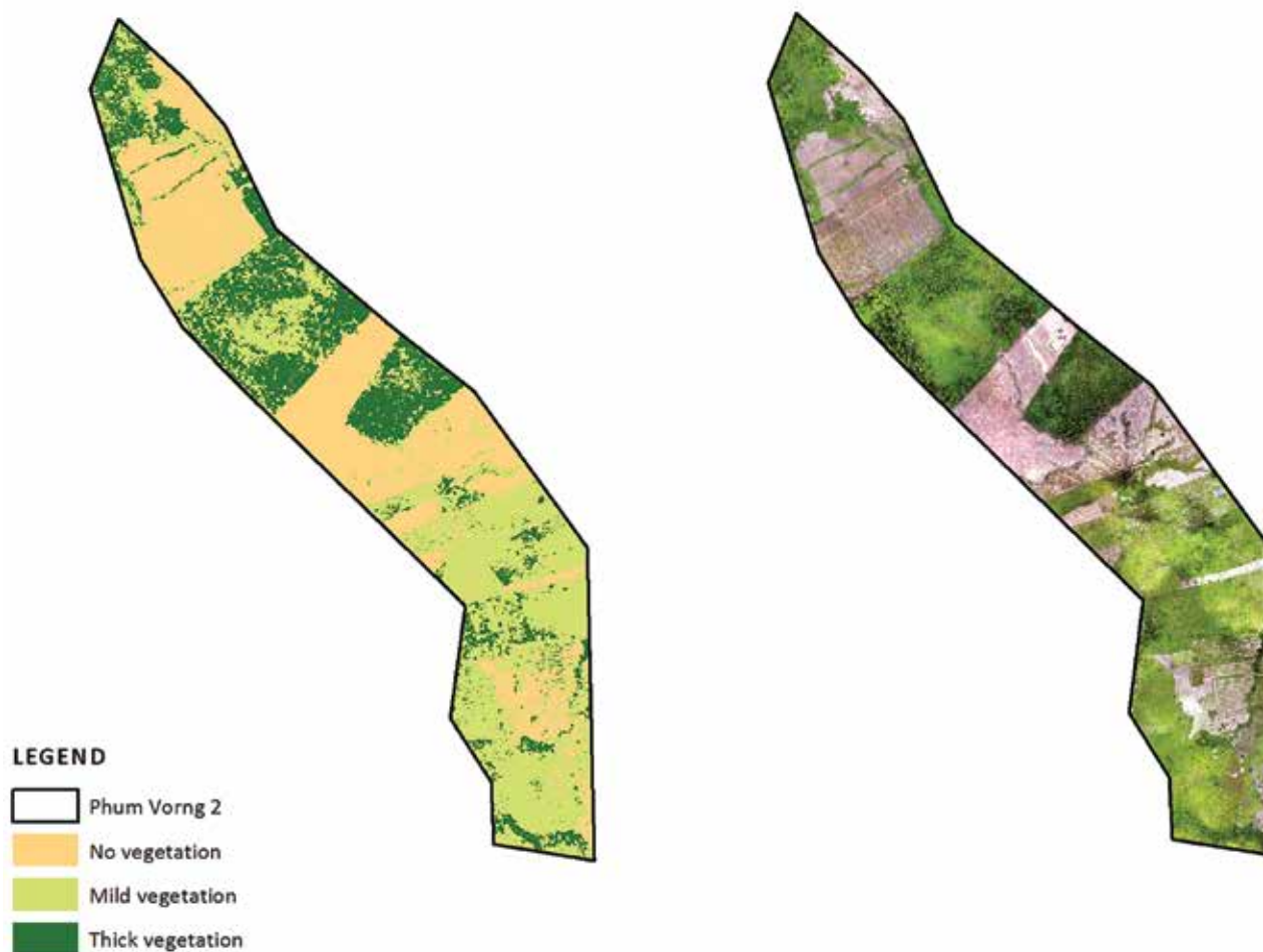
Figure 3. Sample drone images of a battle area clearance site in Northeast Cambodia where the UAV maps replaced the satellite base map and vegetation analyses, divided into three categories.
