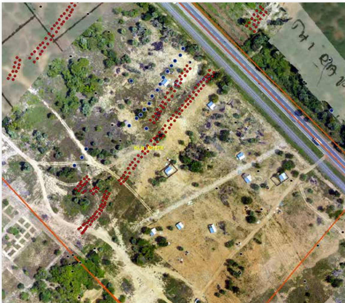
Figure 3. A georeferenced orthomosaic created when using the drone to map large areas. 701 photos have been merged into one. Cleared mines are displayed as red (anti-personnel mines) and blue (anti-tank mines) dots. Image courtesy of The HALO Trust.
