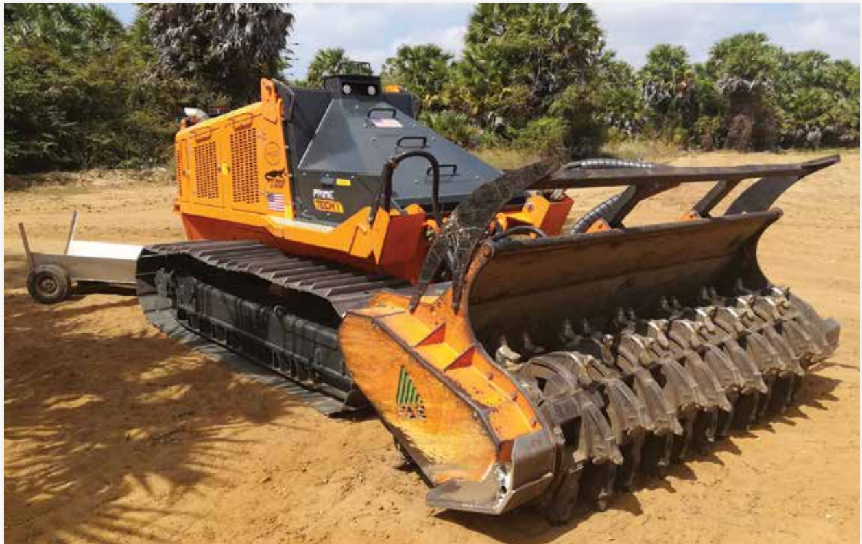
The PrimeTech PT-300 D:Mine tiller. Aerial photos enable proactive deployment into areas that are best suited for certain assets. Image courtesy of The HALO Trust.
