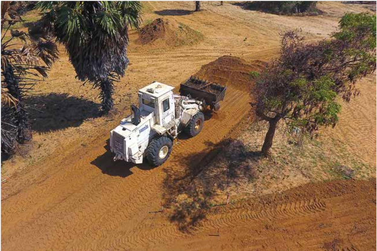
A Case 721C Wheel Loader drops contaminated soil in a marked inspection lane. Aerial photos enable proactive deployment into areas that are best suited for certain assets.
