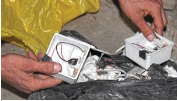
IS anti-lift firing systems. Images courtesy of Terrogence.
