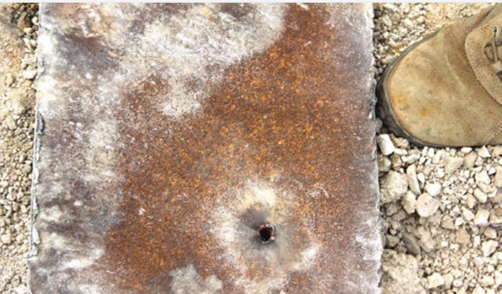
Exit hole in 40-mm thick steel plate from the 35-ml NMD shaped charge.
