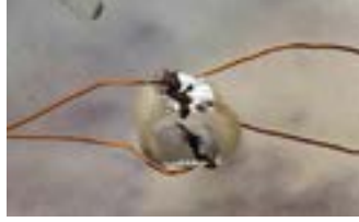
Image 6. A typical crush wire contact. Several dozen switches like this may be present on lengths of lacquered wire up to 10 m in length. 7
