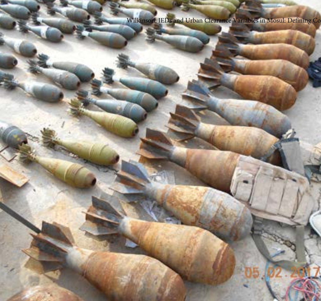
ISIS 210 mm and 120 mm mortar bombs. Note the quality control stickers on the tail sections of the 120 mm mortar bombs (center left).
