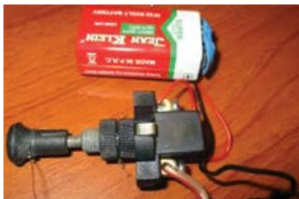
An ISIS “push-pull” toggle switch before and after removal of tape.
