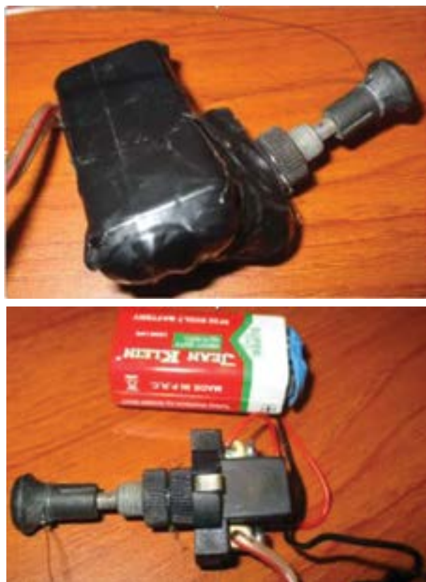
An ISIS “push-pull” toggle switch before and after removal of tape.
