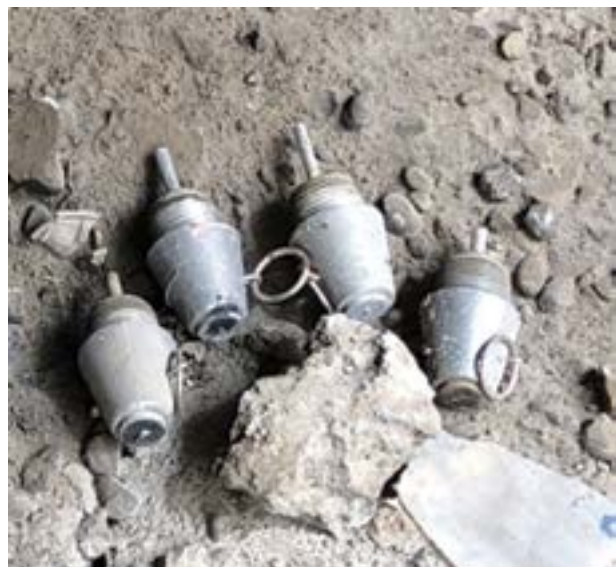
Typical ISIS improvised point detonating fuzes (IDPF).
