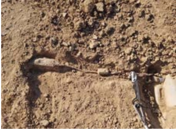
A “j-cutter” positioned prior to semi-remotely cutting a single electrical wire connecting a power source to an IED.
