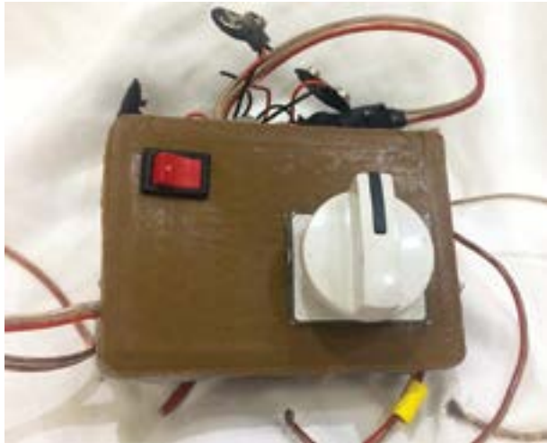
A typical ISIS mechanical timer recovered by UNMAS in west Mosul.
