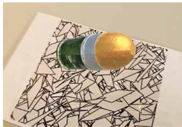
A screenshot from a device viewing a 40 mm rifle grenade up close. Objects appear to users as though they are floating on the marker.
