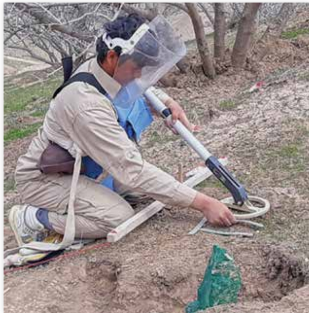
Images 6 (left) and 7 (right). An example of the standard Afghanistan “one man, one lane” (OMOL) technique with a searched area of 1.4 m x 0.3 m, compared to the HALO AIM 2 m breaching technique with a searched area of 2.4 m x 70 cm.
