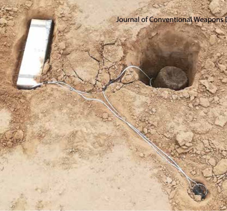
Image 2. A HALO training device shown in a distributed configuration, with the pressure plate, main charge, and battery pack separated from each other and connected with linking wire.
