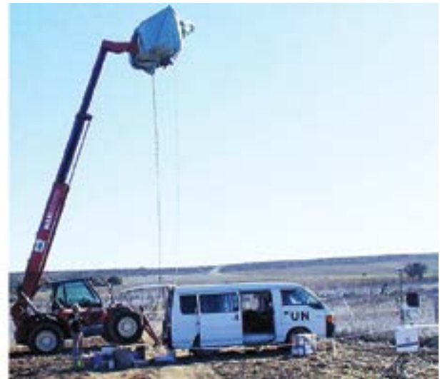
Figure 2. The CLEARFAST thermal/LWIR imaging system over a real minefield in 2005, a precursor to drone capabilities today.
