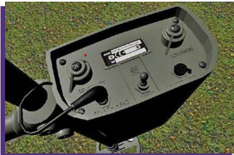
Figure 2. VR model of CEIA MIL-D1 MD metal detector.
