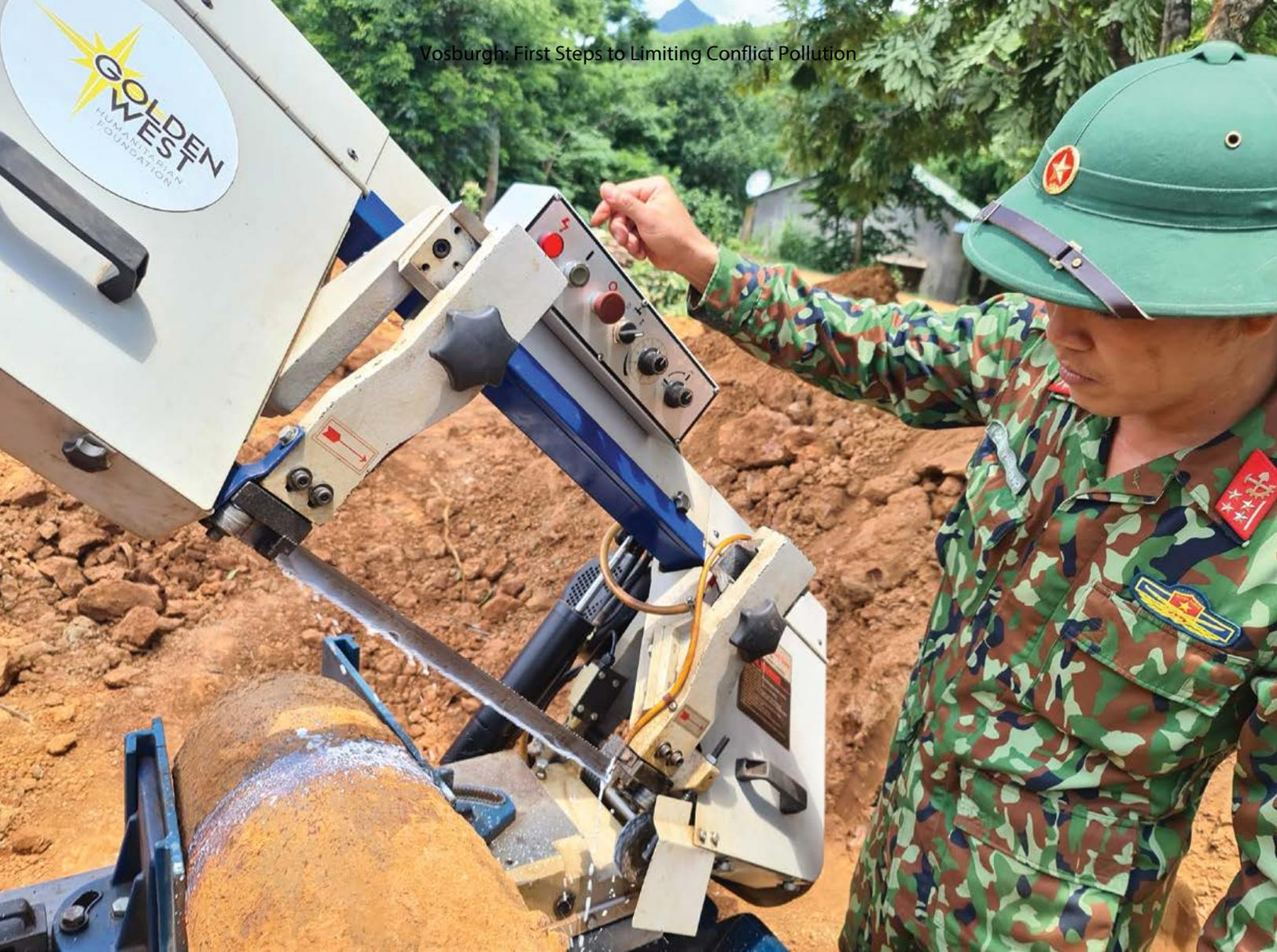
**Image 1.** A PMC Engineer prepares a remote cut on a 500 lb bomb.
