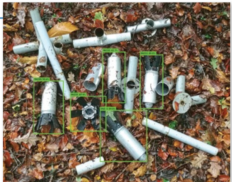
Figure 14. Test on low quality camera with motion blur using real FFE and 9N235/9N210 surrogate (replica) fabricated by Fenix Insight. Courtesy of Adam Harvey.
