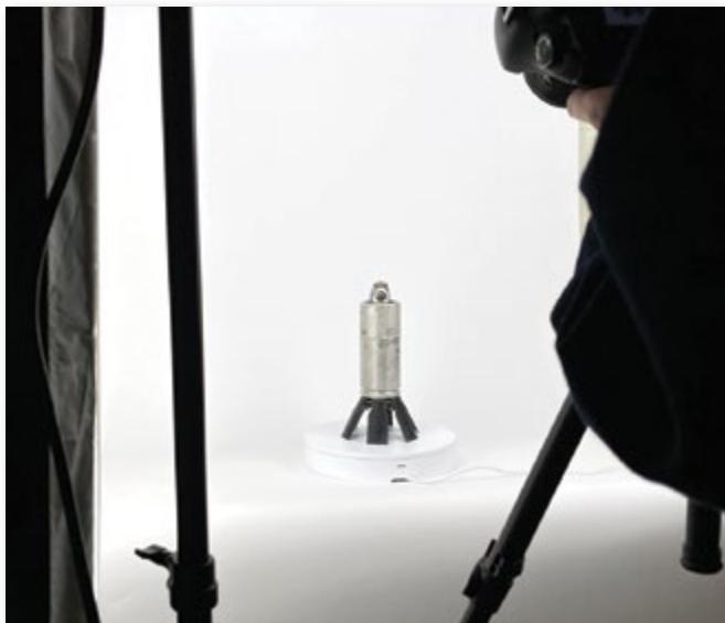
Figure 2. Capturing the original 9N235/9N210 submunition using photogrammetry with an automated turntable and DSLR camera.
