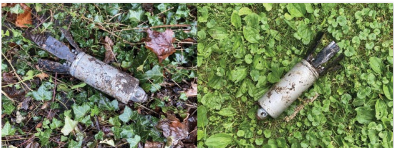
Figures 8 and 9. Real and replica 9N235/9N210 submunitions. Figures courtesy of Adam Harvey.
