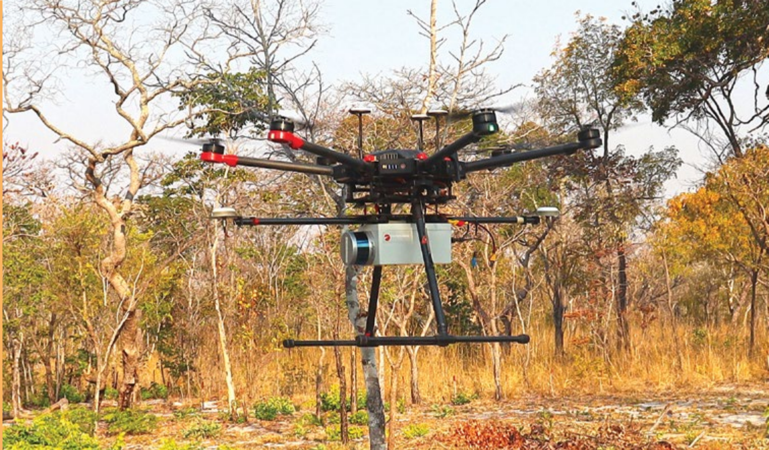
Figure 2. A Routescene LidarPod mounted on a DJI M600 Pro in Angola. Courtesy of Claire Lovelance (The HALO Trust, Angola)
