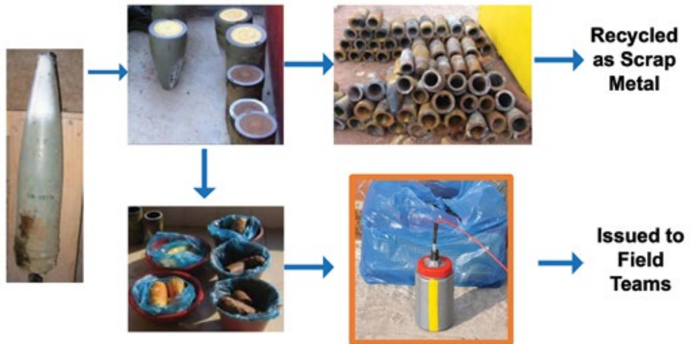
FIGURE 2. Ordnance recycling and water disruptors as a solution for the Philippines, which conceptually illustrates how an EHP program would break down UXO and ERW into recyclable scrap metal and components used to generate water disruptors—a simple tool commonly used by police forces and armies in counter-IED operations. 38
