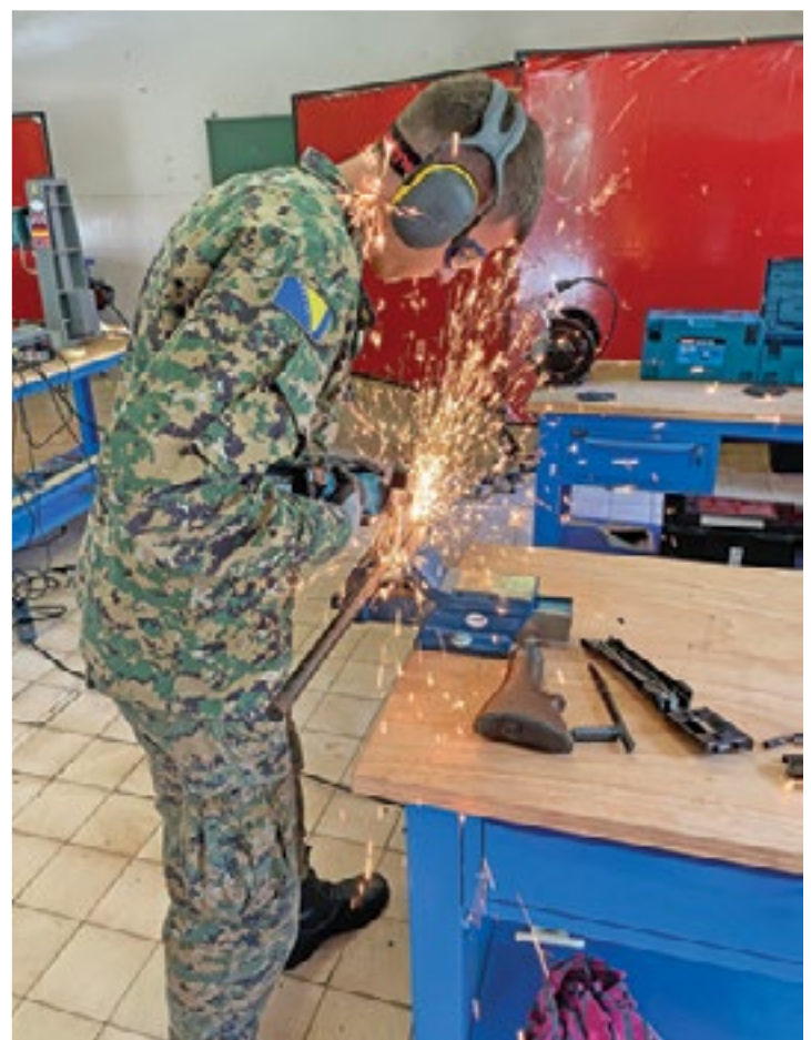
One of the course participants, a member of the AFBiH, in the process of deactivating an MG 34 general-purpose machine gun, in accordance with Regulation (EU) 2018/337. Courtesy of Geir P. Novik.
