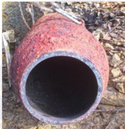
Explosive-free bomb casing following successful burning of explosive filler.
