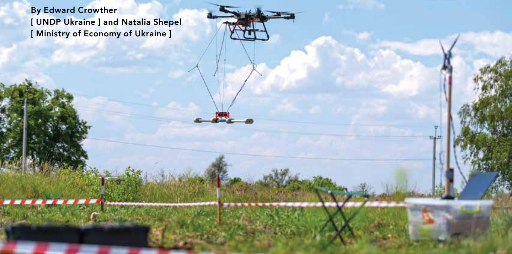
Unmanned aerial vehicle and magnetometer flying over the confirmed hazardous area during Phase II testing, May 2024. Courtesy of Nazarii Mazyliuk/UNDP Ukraine.
